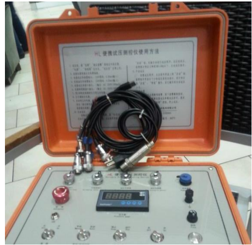
Chen created this device used by oil and natural gas companies in China. The cords connect this device, other units (such as pumps, valves, sensors) and a laptop computer to form a pressure testing system.
